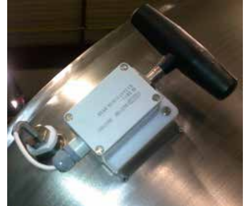
Radio frequency probe for total control of the product temperature
