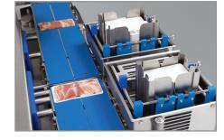
CashinEDGE HS can be set up with a single or dual chambered card dispenser for A and B grade boards. The automatic dispenser places J-boards, including pre-folded boards, under the draft reducing the need for additional labor and handling. J-boards or Carrier boards are loaded from an easily adjustable magazine. All this adds up to superior efficiency and reliability.
